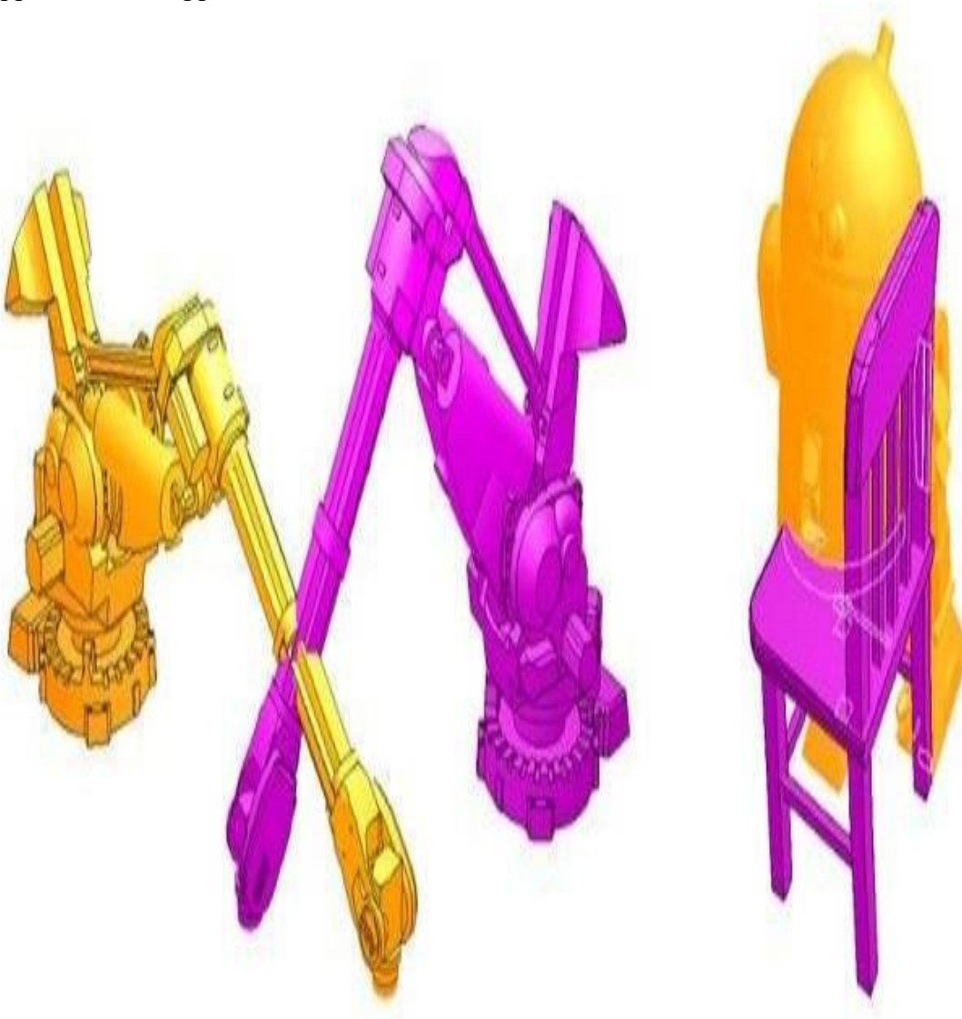
Fig. 3. Collision Detection in Robotic Platform of Coppelia
